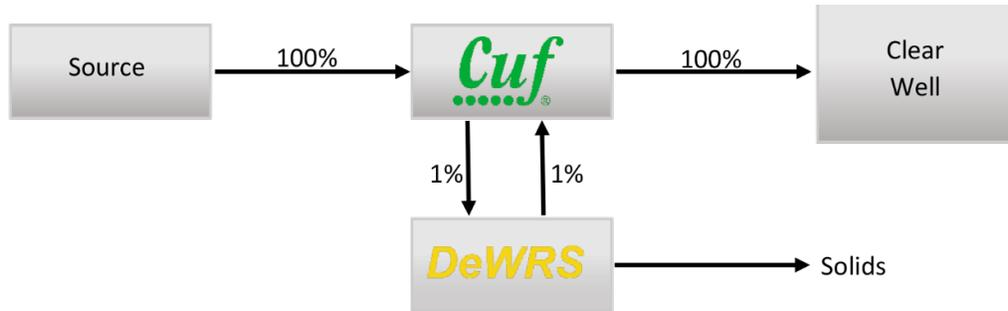
A concentrate blow down is sent to a DeWRS (DeWatering Recovery System) where a 20% solid is achieved without the need for chemical or labor.
